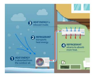
Note: Ductless systems are a cost-effective way to replace inefficient window air conditioning units and replace or displace space heaters and electric baseboard heaters. They can be installed in home additions, new construction, condominiums, and apartments, or to improve temperature control in specific rooms. Ductless systems can even be fit for buildings that currently use ducted forced-air systems.
